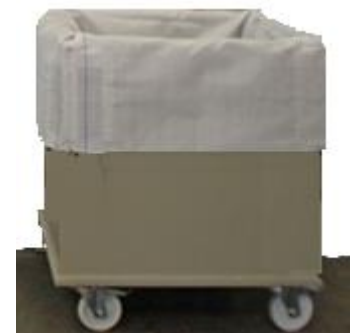
Fig.6 Sludge screening in a large bag, square design
