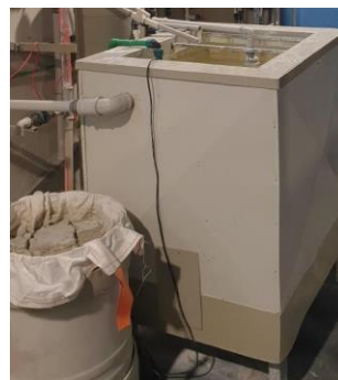
Fig-5 Sludge dewatering large bag in application
