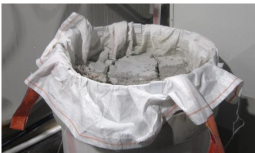
Fig.4 Sludge dewatering large bag in application
